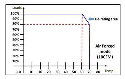
**Note: De-rating Power Output with Temperature**
