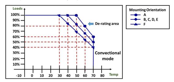
**Note: De-rating Power Output with Temperature**
