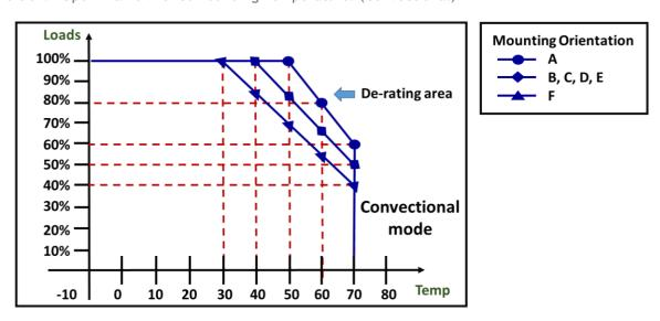
**Note: De-rating Power Output with Temperature**
