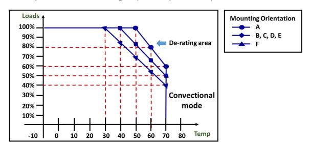
**Note: De-rating Power Output with Temperature**
