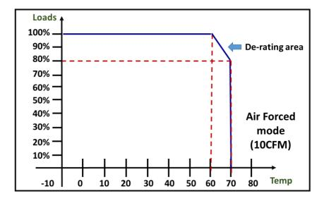
**Note: De-rating Power Output with Temperature**
