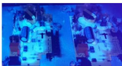
Phihong has well-designed conformal coating processes that is executed by automation equipment rather than traditional manual ways to precisely perform it without leakage to ensure coating quality for any industrial products. This can prevent power supply damage caused by dusts, moisture, or any kinds of unexpected chemical pollutants in the critical application atmosphere to achieve expected robust operation.
