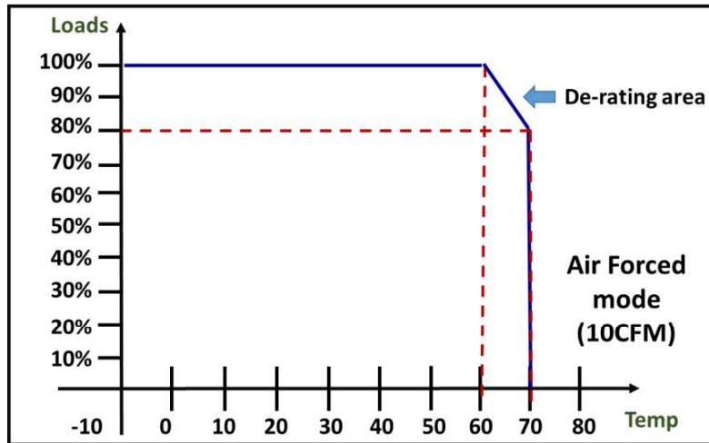
**Note: De-rating Power Output with Temperature**
