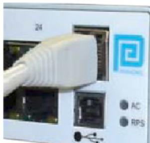
Figure 8: NIC Cable Connected\*
