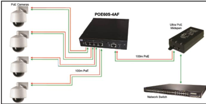
Using standard RJ45 connecting Ethernet cables the POE60S-4AF takes its power from an Ultra or Mega PoE midspan (75W or greater). The output is converted to be IEEE802.3af compatible 15.4W per port. The device can also act as a switch/data repeater by itself. It has an optional 75W DC power adapter, the PSC75U-560 which can power all four ports at 15.4W per port.
