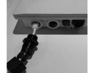
B - Screw the LTGC Body onto the POEO30U/POEO75U Power Injector and tighten the LTGC Body with torque 40-45 in. lbs.(4,5-5,1 Nm)
